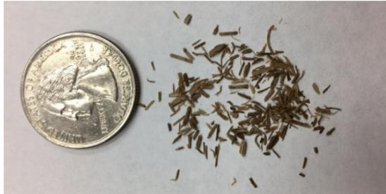
Wood chips in one recommended size for Xtractor
