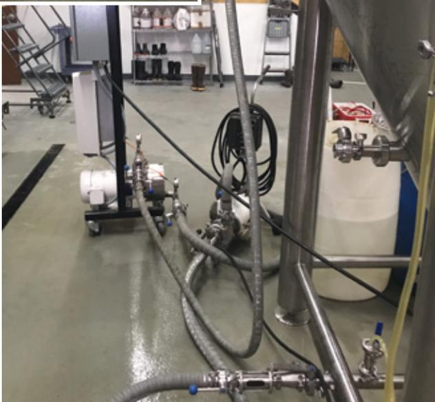
**LEFT: The ShockWave Xtractor takes up a small footprint and is placed on casters so that the brewers at Cabarrus Brewing Company can easily move it around to different tanks in the brewhouse. Photo courtesy of Cabarrus Brewing Company.**
